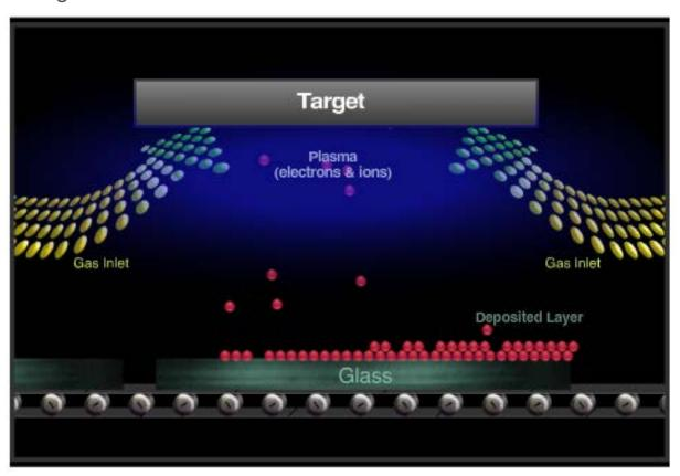
The substrate (glass) enters the coater, gas is then pumped in hitting the targets to create plasma which is then deposited on the glass.
