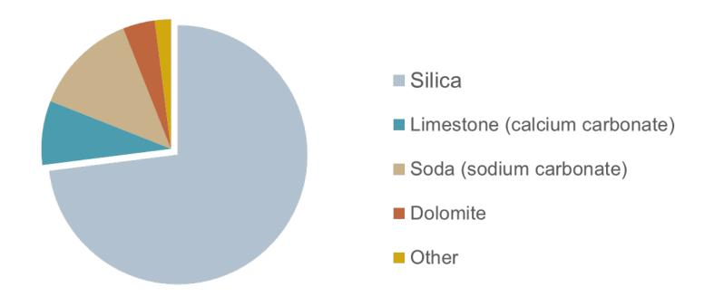
Silica is the most common constituent of sand and is the primary building block of float glass composition.
