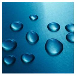
Water beads on spray-on organic coatings, which wear off over time
